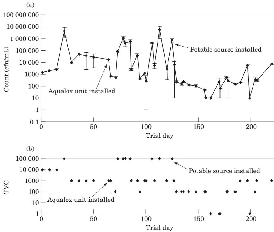
Figure 2 Total viable count (TVC) (a) and dip-slide counts (b) for Tower 2.
