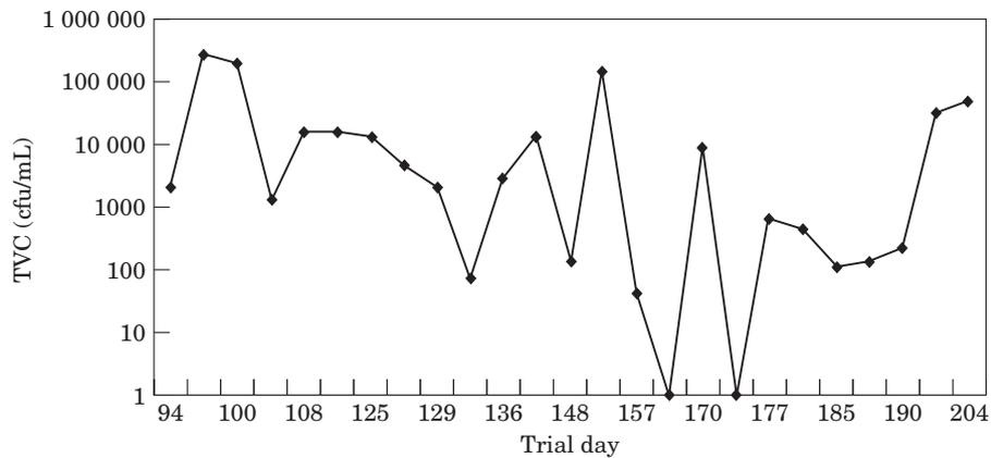
Figure 3 Total viable count (TVC) of non-potable make-up water for Tower 2.
