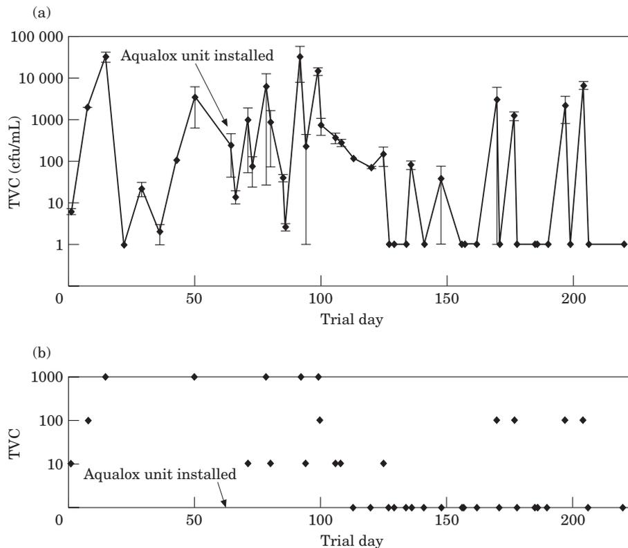
**Figure 1** Total viable count (TVC) (a) and dip-slide counts (b) for Tower 1.
